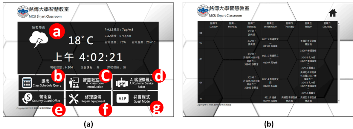
Figure 7. Information board can provide rich classroom context information and interactive functions: In part (a) of this figure, the board shows information including time, weather, class, CO 2 level, PM 2.5 level, indoor temperature, and humidity in portion a. Users can get dynamic classroom schedule, which is shown in part (b), by pressing button b. The functions of button c, d, e, f, g are ‘Smart classroom introduction’, ‘launch a AI chatbot’, ‘Skype call to the security guards’, ‘Skype call to the IT services’, ‘Show welcome message’
