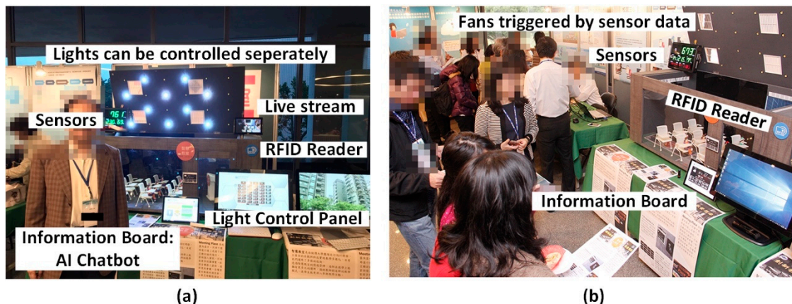
Figure 17. Smart classroom model house demonstration in International Conference on Smart Campus and Exhibition 2018. Most smart classroom functions are re-implemented with Raspberry Pi, Python, and PHP: (a). Lights can be controlled separately with a mobile phone and control panel. A camera toward the whiteboard is live streaming real-time classroom situation; (b) context-aware functions are also implemented, fans on the model house are triggered by CO 2 levels. The RFID reader is used to control the door lock of the model house.
